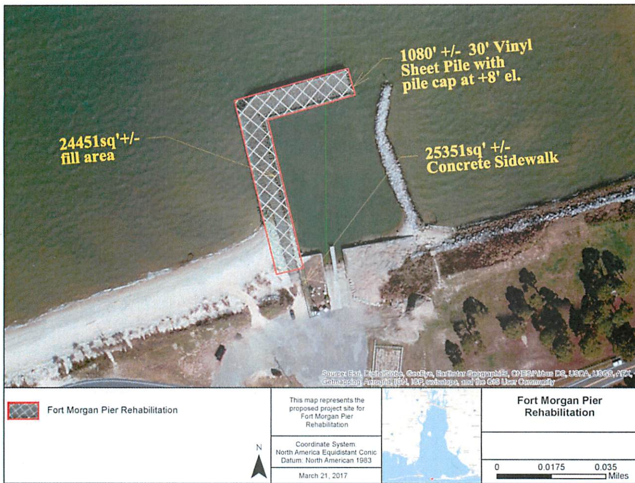
Figure 1. Fort Morgan Pier Rehabilitation Project
