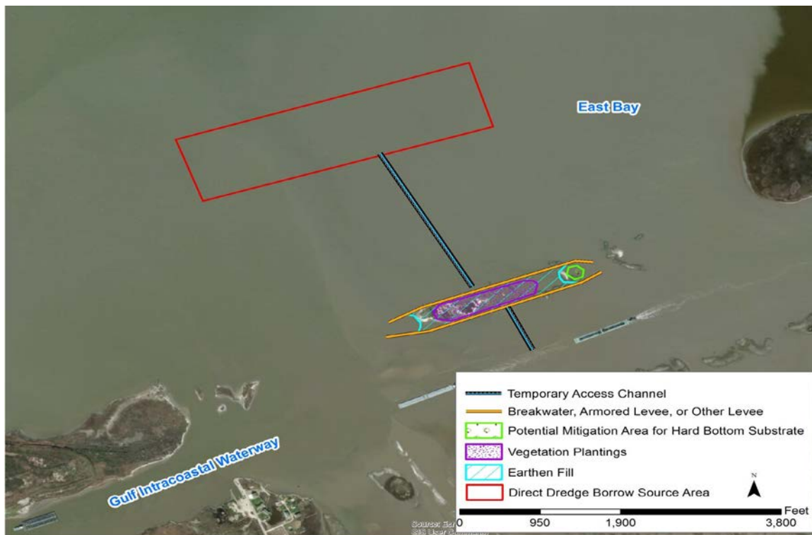
Figure 5. Rollover Bay Island restoration site. Image illustrates the dredge source site, armored shoreline/breakwaters, access channels, and hard bottom mitigation area (image provided by TPWD).
