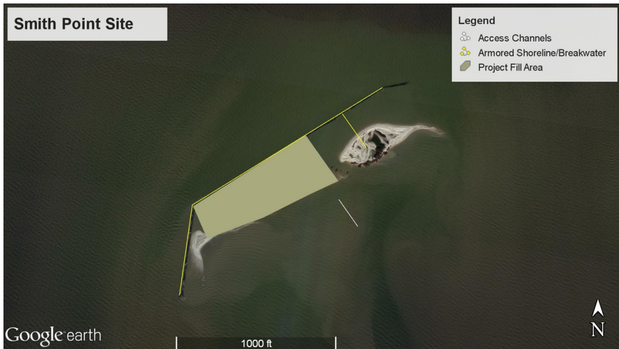
Figure 7. Google image of Smith Point Island with shapefiles provided by TPWD. Image illustrates the armored shoreline/breakwaters, access channels, and the project fill site location (Google Earth, 2016).
