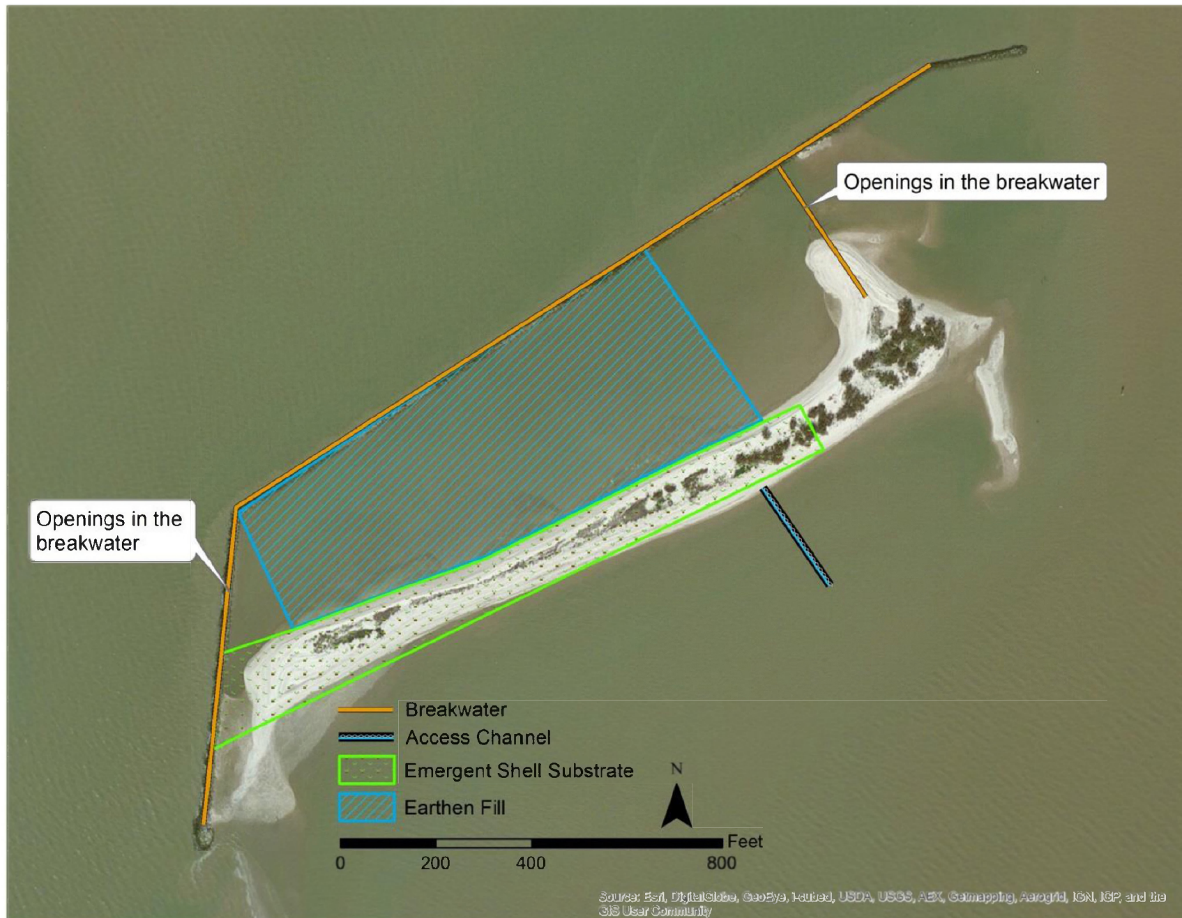
Figure 5. Proposed restoration and protection features for Smith Point Island showing access channel and describing openings in breakwater associated with interior lagoons to allow ingress and egress of tidal waters.
