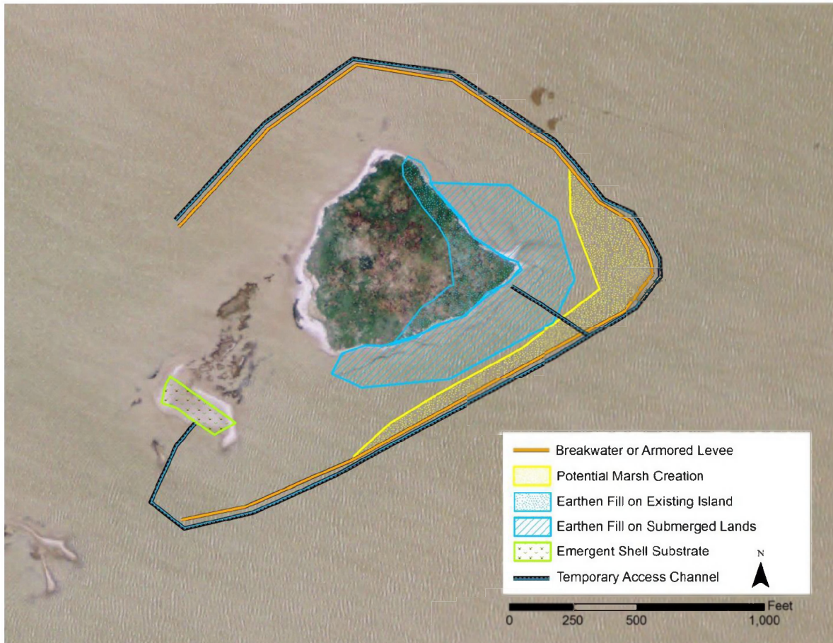
Figure 6. Conceptual drawing of the proposed Dressing Point Island restoration, illustrating the footprint of the breakwater/levee, fill, and emergent shell substrate.
