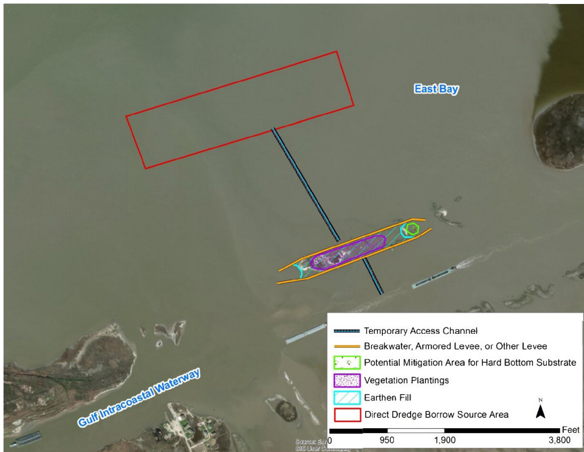
Figure 4. Conceptual drawing of the proposed Rollover Bay Island restoration, illustrating potential temporary access channels, the footprint of the breakwater/levee, fill, and vegetation planting area.
