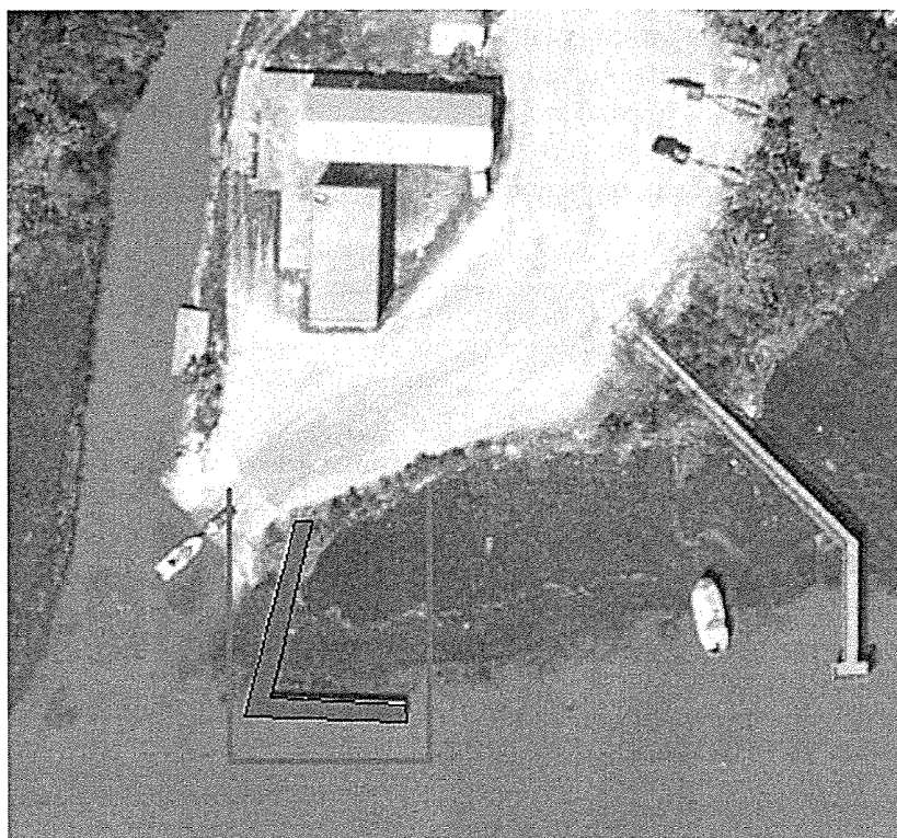
Figure 4. Image of the Waterfront Park improvement site with the dock enhancement (red polygon) and the turbidity curtain (red open rectangle). (©2014, C. Robertson, FL DEP)
