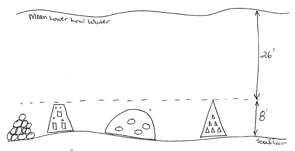
Material: concrete and rock rubble Pre-fabricute reef modules
