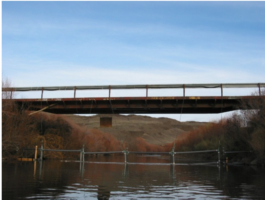
Figure 3. Oasis Road Bridge dual loop pass through PIT detection array.
