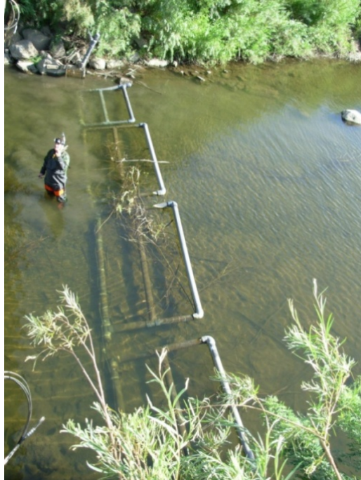
Figure 4. Oasis Road Bridge dual loop pass through PIT detection array showing antenna cable plug-ins near the bottom of the river, and the new, free-floating design.
