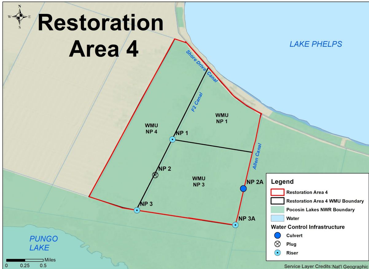
Figure A-32. Restoration Area 4 (RA 4) restoration infrastructure and current and potential water management units (WMUs).
