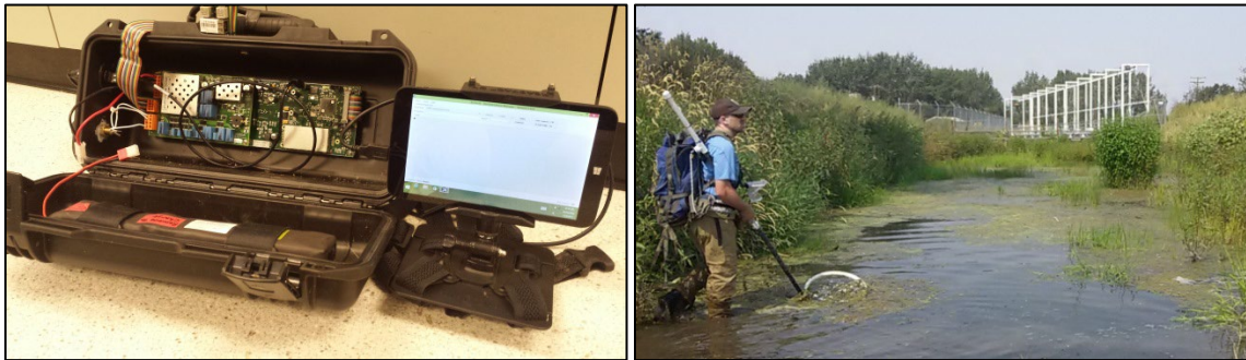
Figure 7. An IS1001ACN-based mobile PITpack reader. (A) The PITpack reader is comprised of a waterproof Pelican case, a Windows-based tablet mounted in a harness, a detection alarm, and a lithium-ion battery. (B) Scanning a drained Feed Diversion Canal with a PITpack detection wand, 2015.
