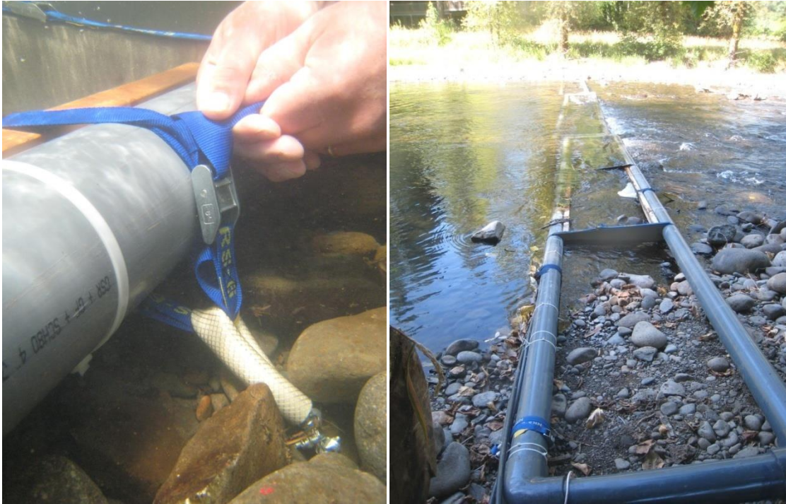
Figure 3. Eagle Creek Mouth (ECM) detection array and stream bottom anchoring system during base flows.
