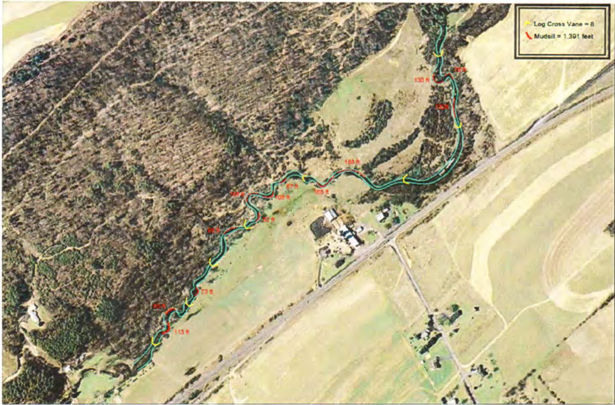
Figure 3. Stream habitat enhancements to Musser Run. Approximately 8 log cross vane (yellow) and 1.3 ft of mudsills (red) will be placed in Musser Run to improve stream habitat.
