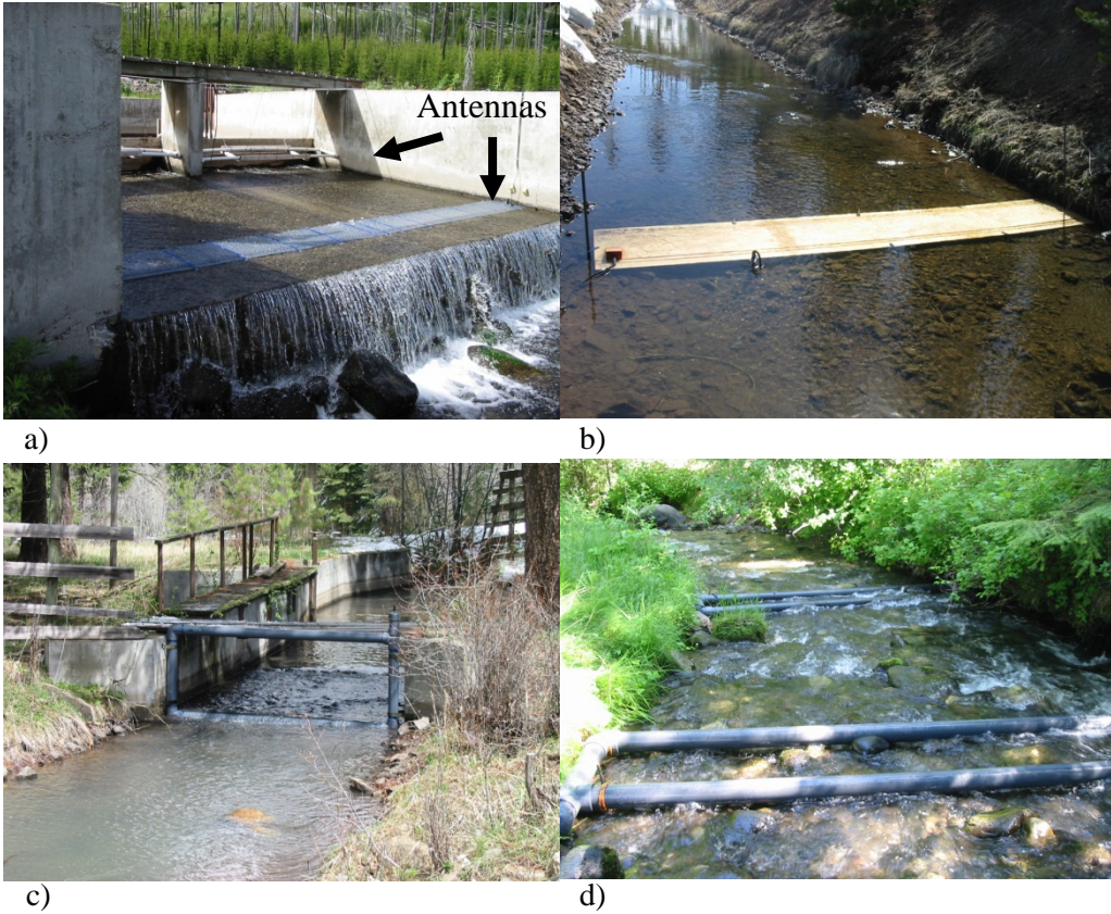
Figure 12. Antennas installed in 2007 - a) Big Sheep Creek diversion flat panels and upper antennas; b) upstream of Salt Creek summit flat panel (wood); c) Antenna in the WVIC just below where McCully Creek goes under the canal; d) McCully Creek antennas upstream of the WVIC.
