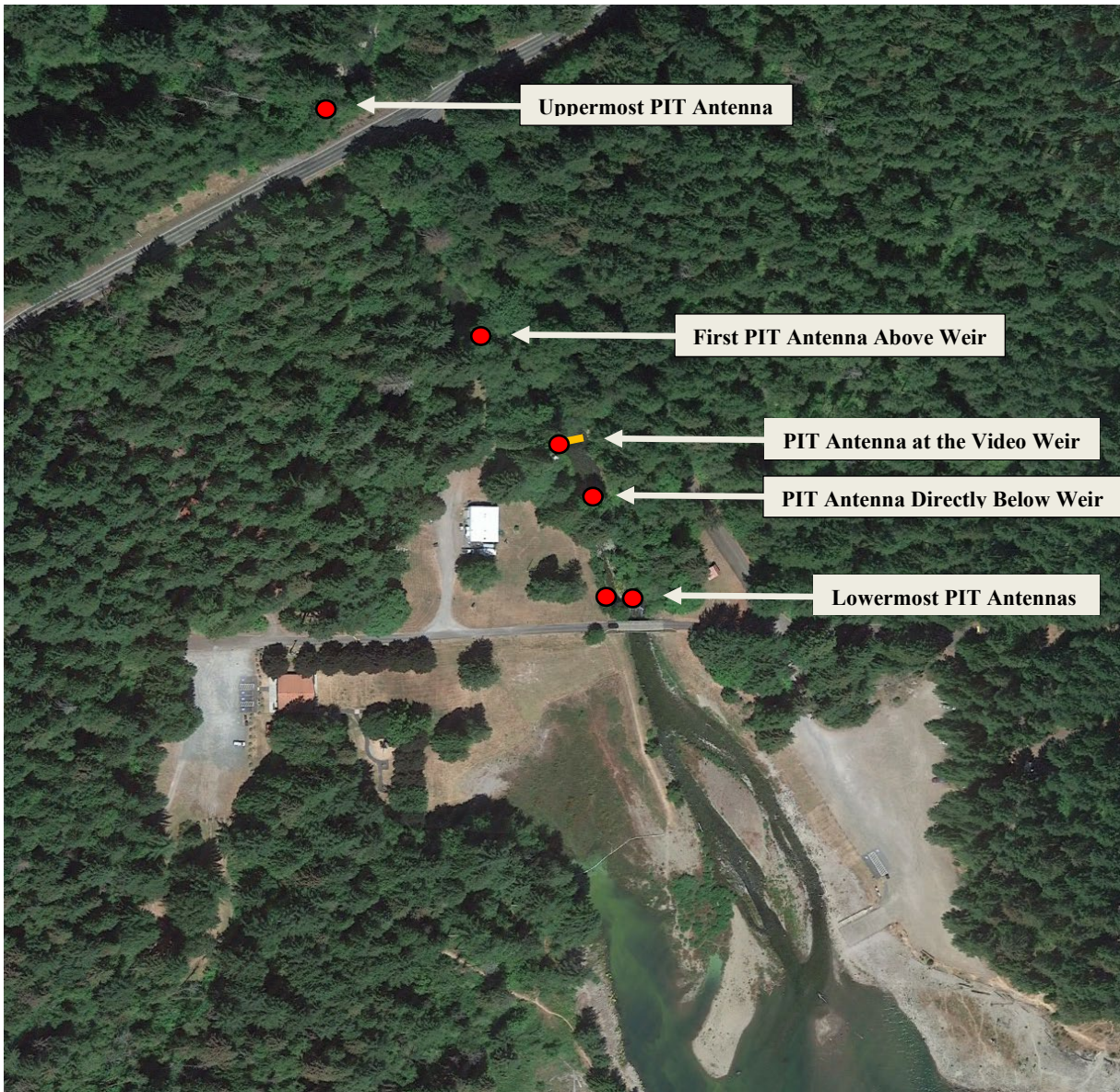
Figure 5. Aerial photo depicting locations of PIT antennas in Cougar Creek upstream and downstream of the weir during 2021 (Google Earth imagery date: July 25, 2021).
