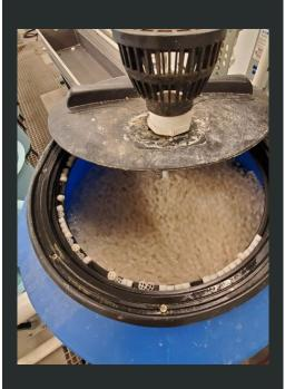
Keep up with your water quality! Cal Fraser recognized some inefficiencies with the bio-filtration cycle. This bio-media appeared to be rolling the way it should. However, below the surface ½ of the media was connected by a build up of calcium carbonate. The calcium carbonate built up over the last few trials from heating the hard water common to the BFTC.
