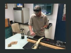
Zack Conley working on the extruder screws for maintenance in the feed manufacturing building. Taking note of the order the screw heads are taken off, the twin drive barrel requires both sets to be paired exactly.
