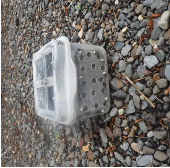
Appendix Figure 1. Design of the containers in which larval lamprey were held during the growth experiment in the Umatilla River from 17 July to 24 August 2022.
