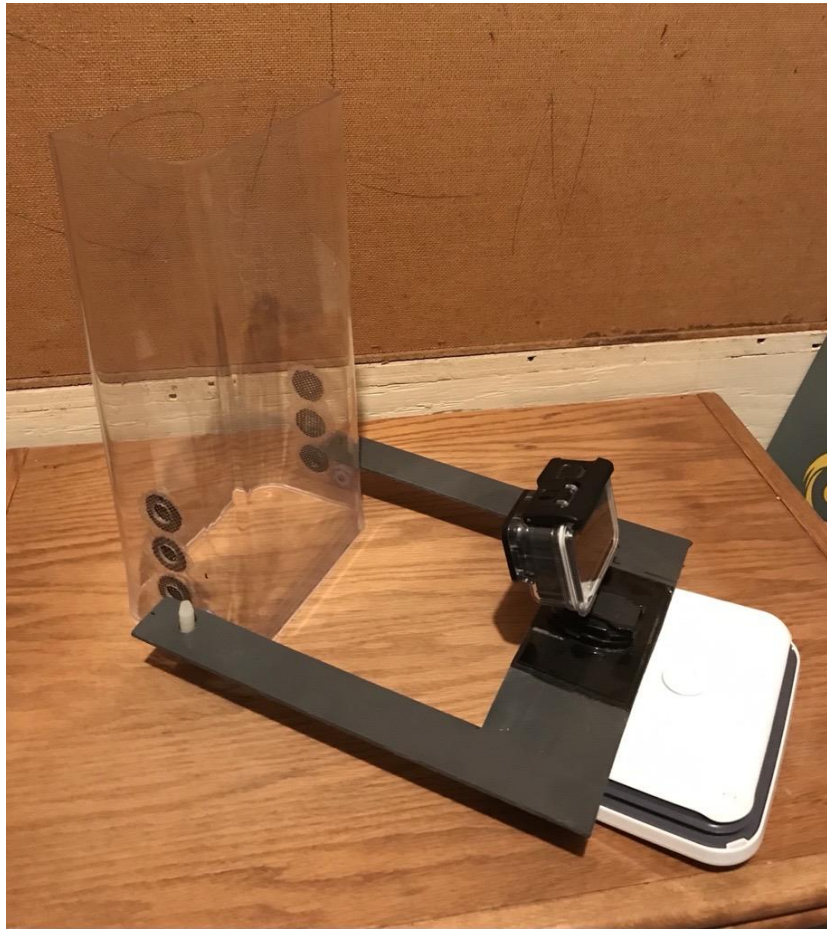
Appendix Figure 2. Design of the plexiglass chamber and GoPro used in the burrowing experiment in the Umatilla River on 27 and 28 July 2022.
