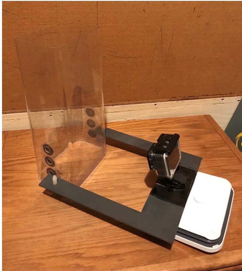
Appendix Figure 2. Design of the plexiglass chamber and GoPro used in the burrowing experiment in the Umatilla River on 4 and 5 August 2021.
