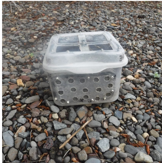
Appendix Figure 1. Design of the containers in which larval lamprey were held during the rowth experiment in the Umatilla River from 19 July to 30 August 2021.
