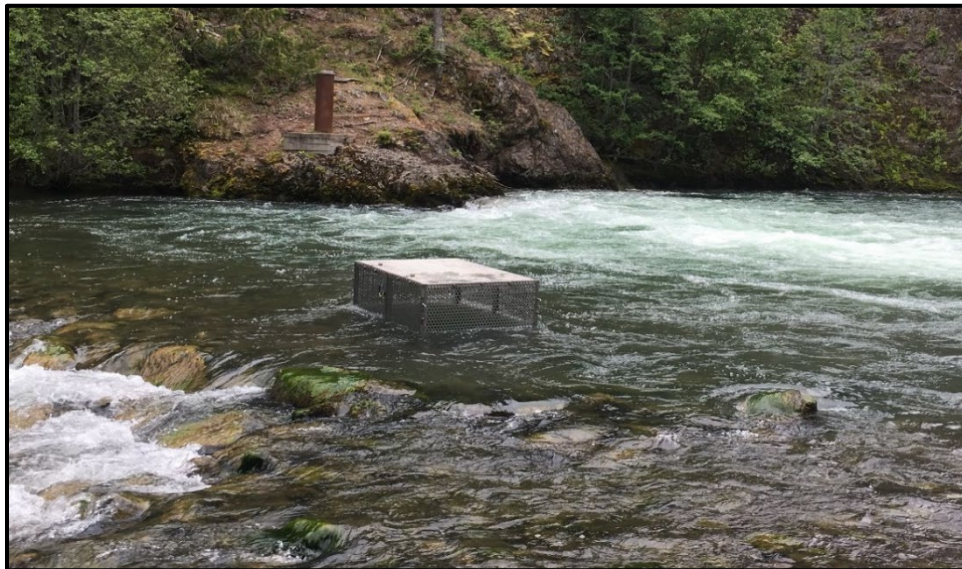
Figure 4. Stainless steel pen (0.9 m x 1.2 m x 1.8 m) used for holding Bull Trout after collection and before rapid response genetic testing and transport to natal watershed.
