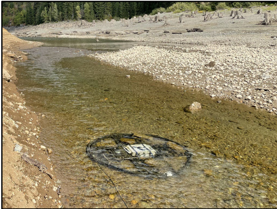
Figure 3. Example of a submersible antenna monitoring the movement of PIT-tagged Bull Trout.
