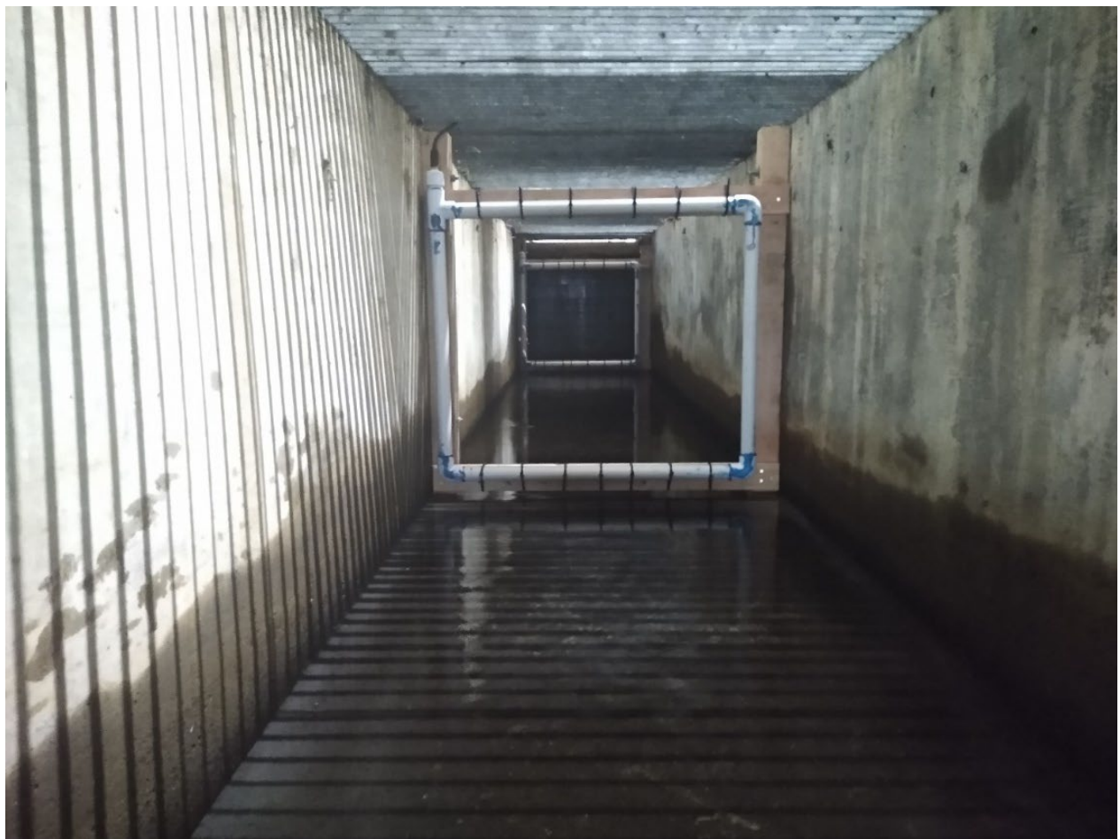
Figure 2. FDX PIT tag antenna array located in secondary bypass channel, immediately downstream from sampling Unit #1.
