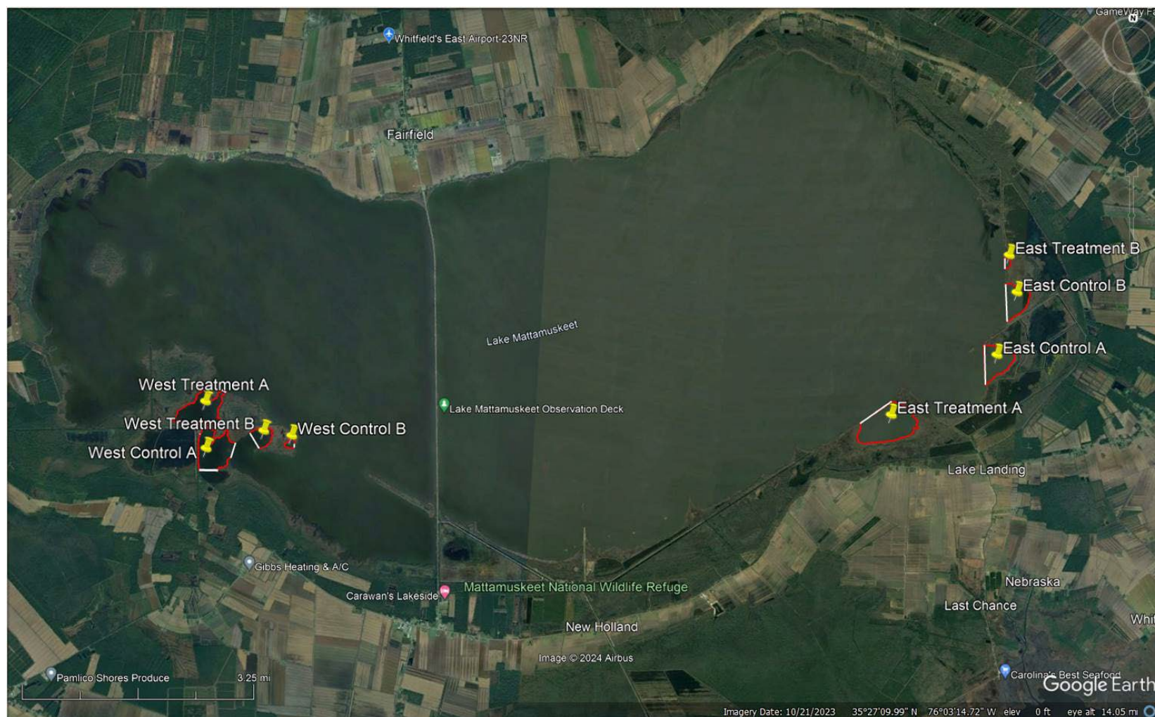
Figure 2: An aerial image of Lake Mattamuskeet and the proposed sites for treatment with Lake Guard® Oxy and control sites. The red lines depict Treatment and Control sites with white lines denoting turbidity curtain locations. This image was provided by BlueGreen Water Technologies on March 2, 2024.
