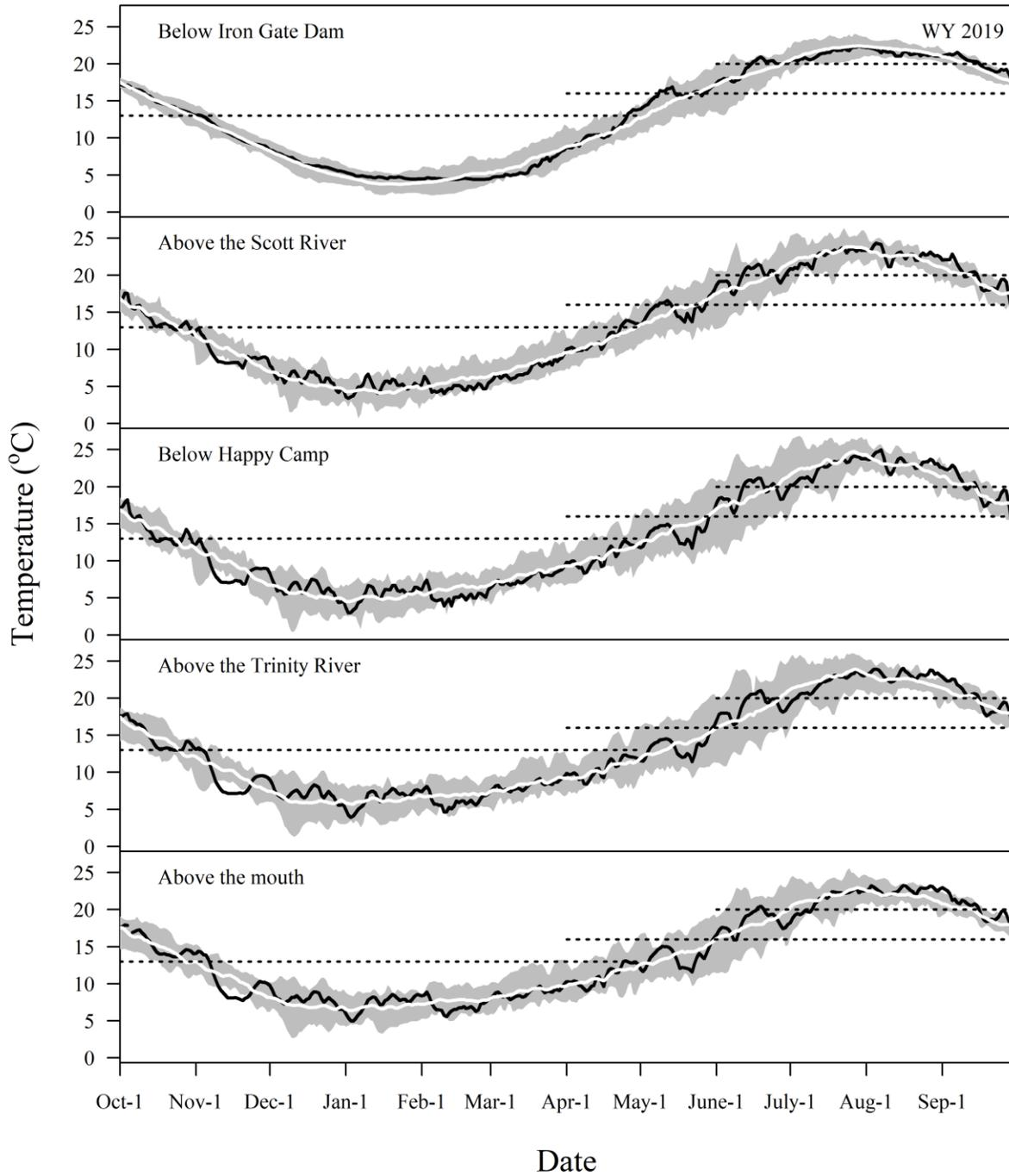
Figure 4. Seven-day average daily maximum temperature (7DADM) at focal Klamath River monitoring sites during water year (WY) 2019 (i.e., October 1, 2018 – September 30, 2019), with historical summaries from WYs 2001 to 2018. Black line = 7DADM water temperatures in 2019; white line = average historical 7DADM for each day of the year; gray polygon = range of historical 7DADM for each day of the year; black dotted line = EPA Pacific Northwest water temperature criteria.
