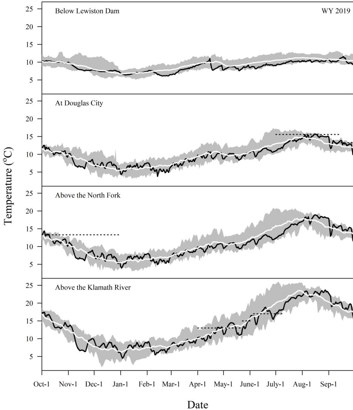
Figure 2. Daily mean water temperatures at focal Trinity River monitoring locations in water year (WY) 2019 (i.e., October 1, 2018 – September 30, 2019), with historical summaries from WYs 2002 to 2018. Black line = daily mean water temperatures in 2019; white line = average historical daily mean for each day of the year; gray polygon = range of historical daily mean water temperatures for each day of the year; black dotted line = water temperature criteria.
