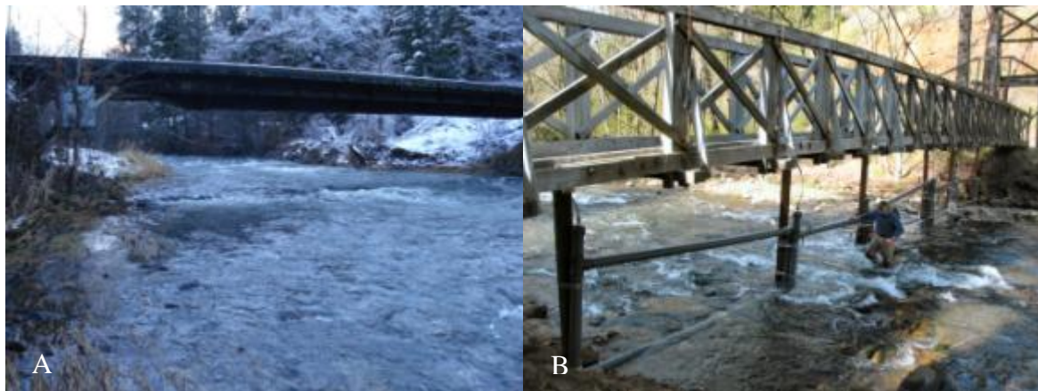
Figure I-11. The Kiwanis Camp Bridge (KCB) passive instream antenna showing pass over antenna configuration (A) and original pass through antenna configuration (B).
