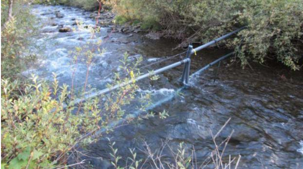
Figure I-3. Bear Creek (WW2) PIA spanning the South Fork Walla Walla River. Antenna 1 and 2 are located on the left and right, respectively.
