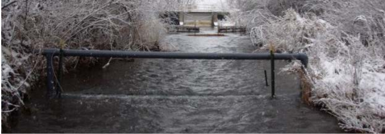
Figure I-14. Downstream view of the upper Yellowhawk Creek (YHC) passive instream antenna.
