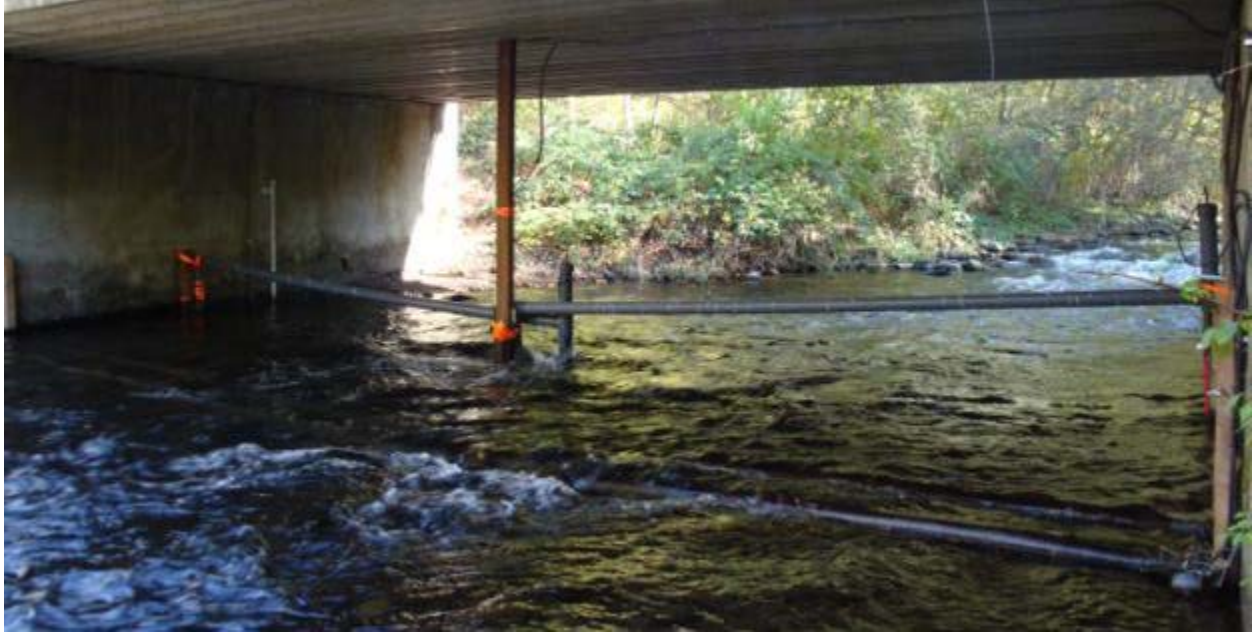
Figure I-4. Harris Park Bridge (WW1) PIA showing pass through antennas (upstream) and pass over antennas (downstream).
