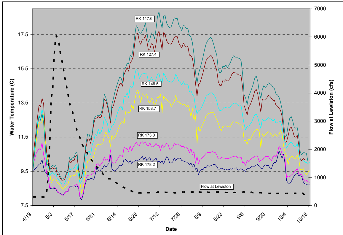
Figure 5. Average daily water temperatures of the Trinity River from Lewiston gage (RK 178.2) to Pear Tree Gulch gage (RK 117.6), USFWS data, 2002.
