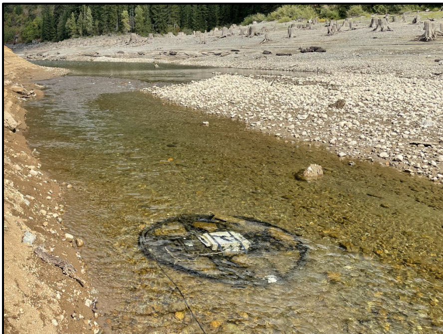
Figure 4. Example of a submersible PIT antenna.
