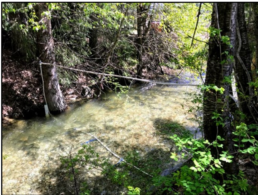
Figure 3. Example of a pass-through PIT antenna.
