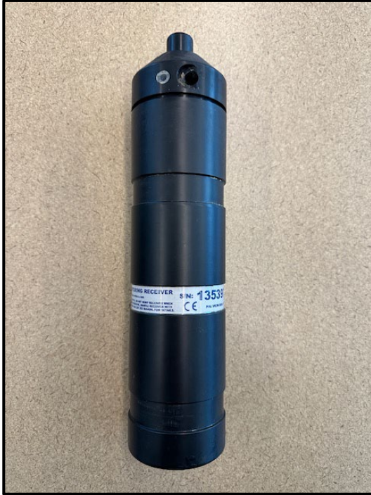
Figure 5. Example of an acoustic receiver deployed in Keechelus Reservoir in 2024.
