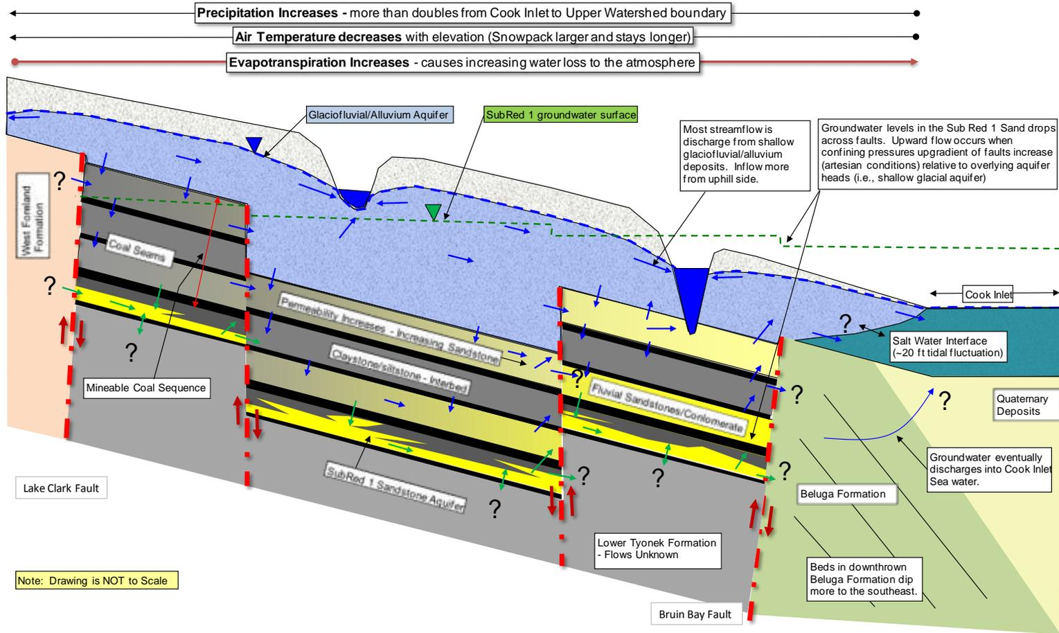
**Figure E-3. Conceptual flow model for the Chuitna watershed**
