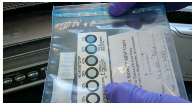
Figure1. DBS Kit containing Whatman 903 ® Filter Card, silica gel desiccant sachet and a Humonitor ® strip
