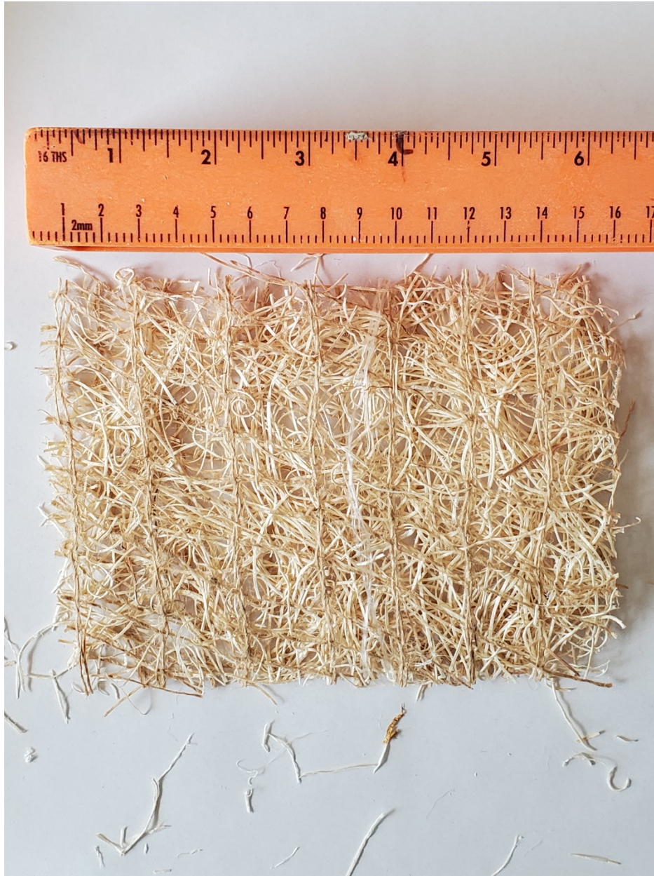
Figure 5 Curlex III. Aspen excelsior contains FibreNet netting on two sides (1in * 0.5 in) jute with moveable joints. Slopes \leq 1H:1V , Channels 2.5 lb/ft 2 (120 Pa) shear stress, 10.0 ft/s (3.1 m/s) velocity. True biodegradable, seed free. Mowable in 90 days. Wildlife friendly.
