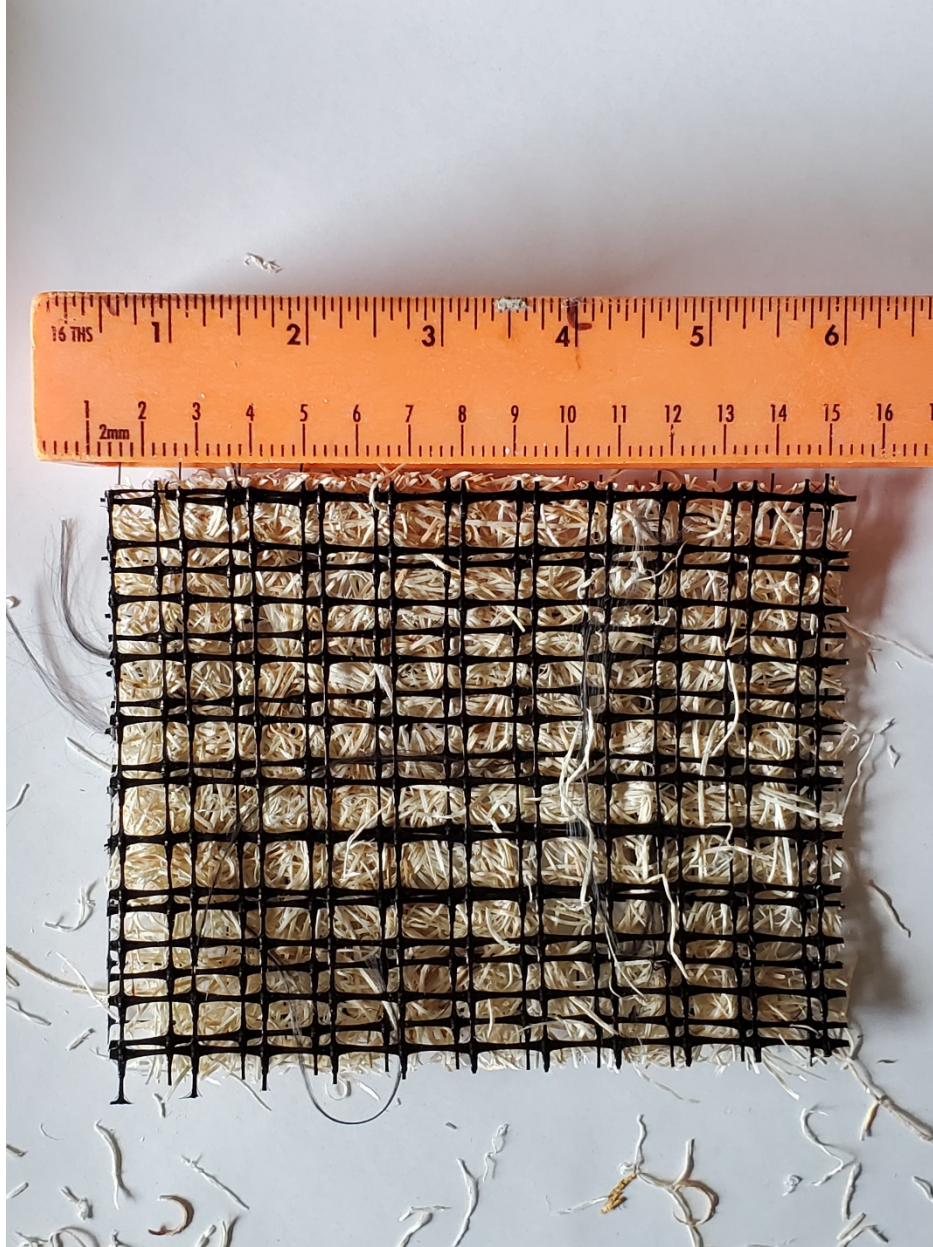
Figure 7 Trinet Curlex side 1. Aspen excelsior contains standard polypropylene netting on both sides (0.5 in * 0.5 in) welded joints, heavy duty, and UV stabilized. Slopes \leq 5H:1V , Channels 13 lb/ft 2 (622 Pa) shear stress, 20.0 ft/s (6.1 m/s) velocity. Seed free Permanent reinforcement, also available in natural straw/coconut, natural coconut, Recyclex synthetic fibers with the same netting. Not wildlife friendly.
