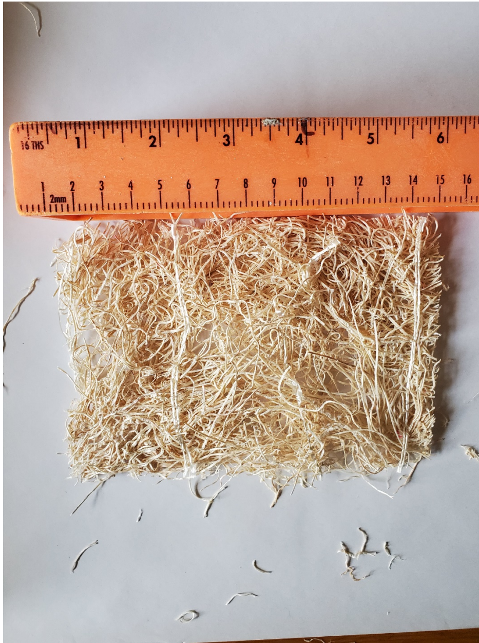
Figure 2 Curlex NetFree. Aspen excelsior contains no netting. Slopes \leq 3H:1V , Channels 1.0 lb/ft 2 (48 Pa) shear stress, 3.0 ft/s (0.9 m/s) velocity. True biodegradable, seed free. Wildlife friendly.
