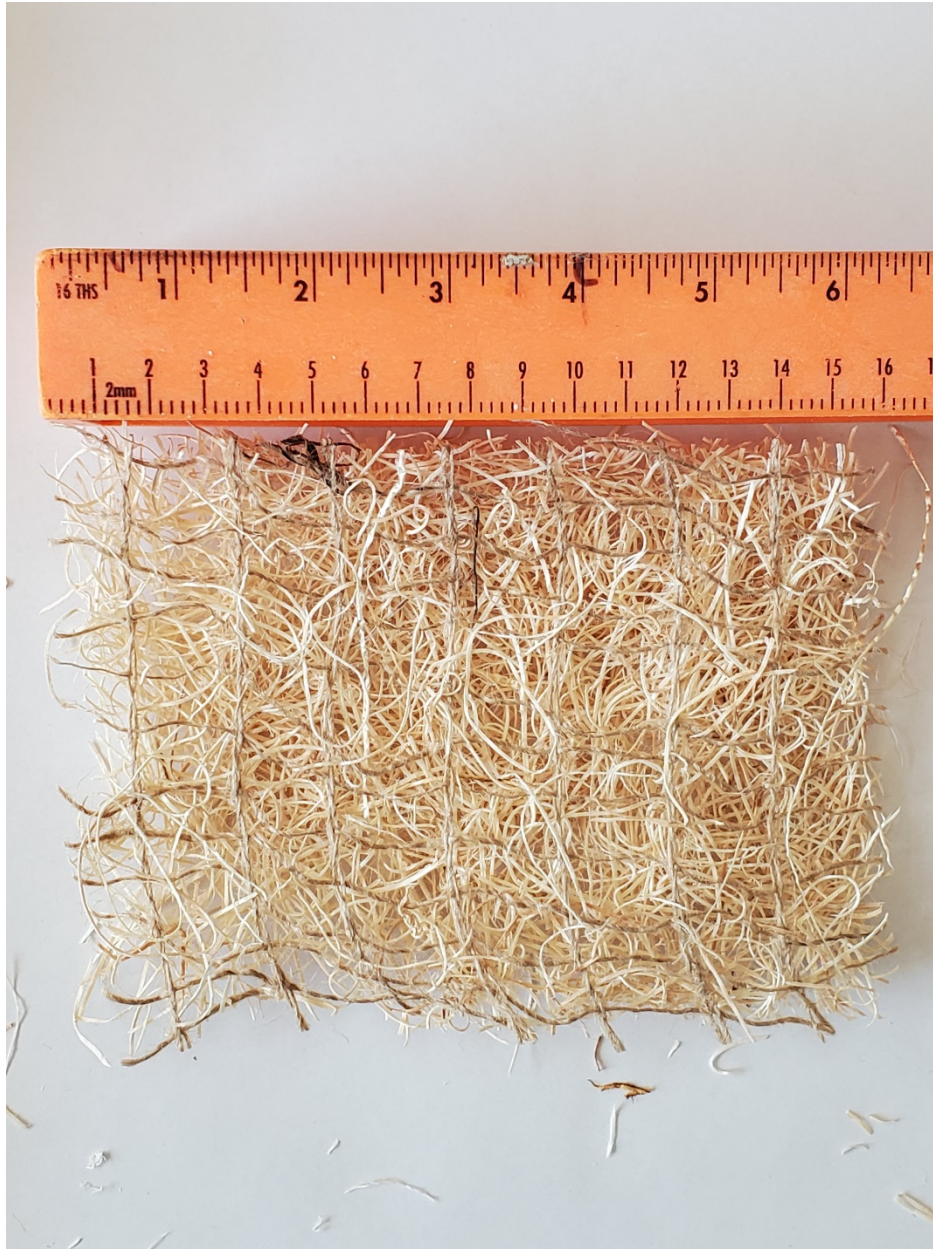
Figure 4 Curlex II. Aspen excelsior contains FibreNet netting on two sides (1in * 0.5 in) jute with moveable joints. Slopes \leq 1.5H:1V, Channels 2.25 lb/ft 2 (108 Pa) shear stress, 9.0 ft/s (2.7 m/s) velocity. True biodegradable, seed free. Mowable in 90 days. Wildlife friendly.
