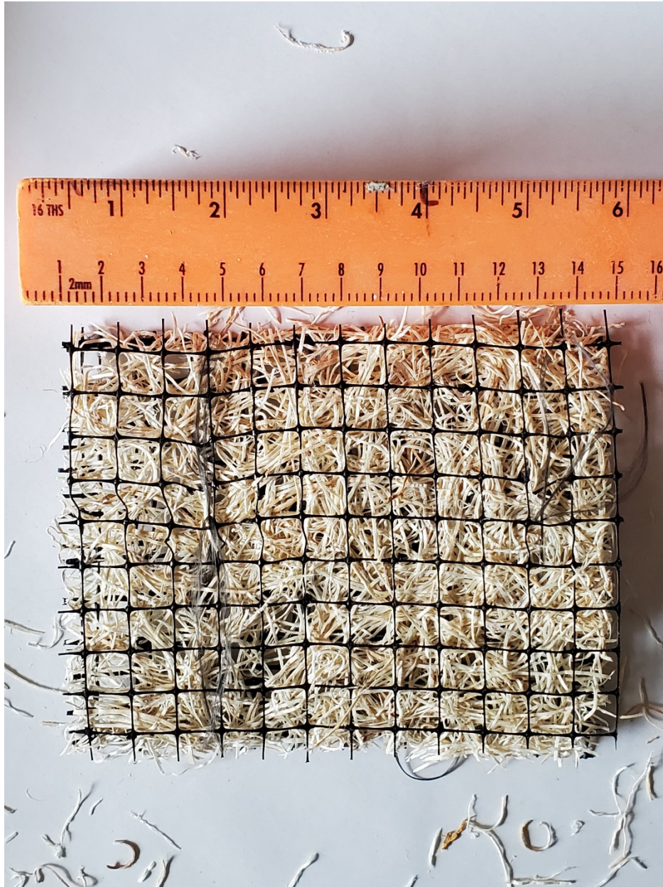
Figure 8 Trinet Curlex side 2. Aspen excelsior contains standard polypropylene netting on both sides (0.5 in * 0.5 in) welded joints, heavy duty, and UV stabilized. Slopes \leq 5H:1V , Channels 13 lb/ft 2 (622 Pa) shear stress, 20.0 ft/s (6.1 m/s) velocity. Seed free Permanent reinforcement, also available in natural straw/coconut, natural coconut, Recyclax synthetic fibers with the same netting. Not wildlife friendly.
