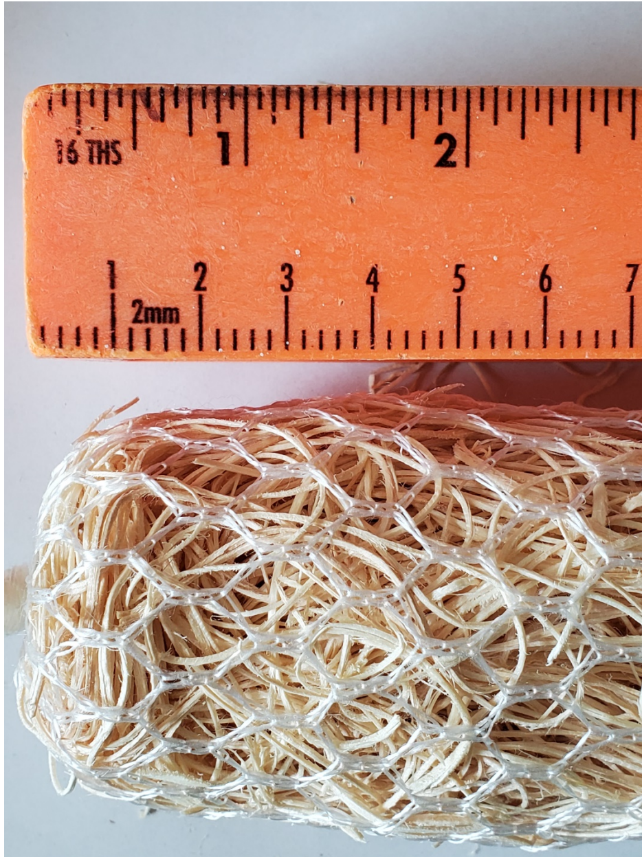
Figure 9 Curlex sediment log. Aspen excelsior covered in open weave containment fabric on both sides (0.5 in hexagon) open weave joints. Filters and reduces hydraulic energy and sediment runoff. Available in 20, 12, 9, 6 inch or customizable lengths. Seed free, ≤ 24 months lifespan. Open weave mesh makes this less risky to wildlife.
