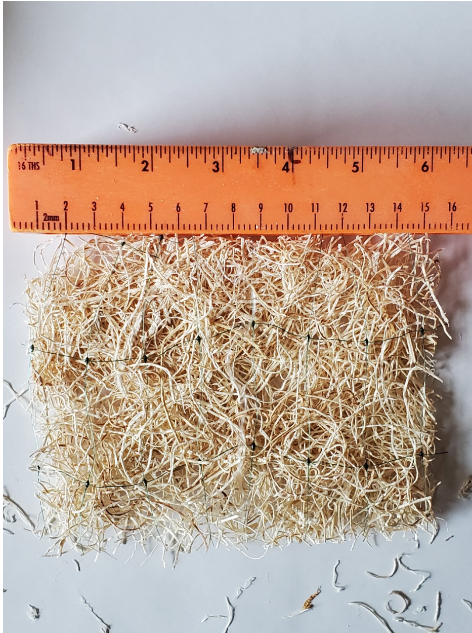
Figure 6 Curlex I. Aspen excelsior contains standard polypropylene netting on one side (2 in * 1 in) welded joints, oxo-biodegrader, and UV additives. Slopes \leq 2H:1V , Channels 1.75 lb/ft 2 (84 Pa) shear stress, 7.0 ft/s (2.1 m/s) velocity. Seed free. Larger mesh size makes this less risky to snakes, but does not meet criteria for fully wildlife friendly.
