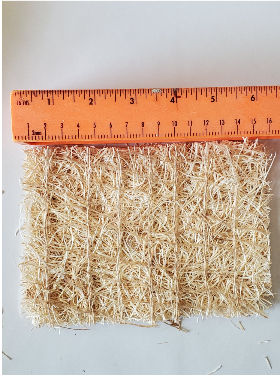
Figure 3 Curlex I. Aspen excelsior contains FibreNet netting on one side (1in * 0.5 in) jute with moveable joints. Slopes \leq 2H:1V , Channels 1.75 lb/ft 2 (84 Pa) shear stress, 7.0 ft/s (2.1 m/s) velocity. True biodegradable, seed free. Mowable 90 days. Wildlife friendly.
