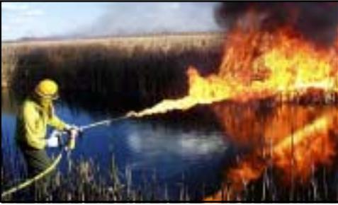
*This "Terra-Torch" is used to cross water barriers such as ditches. It also enables fire crews to work without having to wade in marsh muck.*
